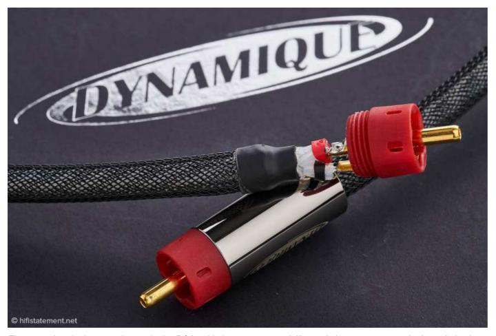
The ground and minus conductors in the RCA cable have a narrow, deliberately low-mass contact in the red plastic.
